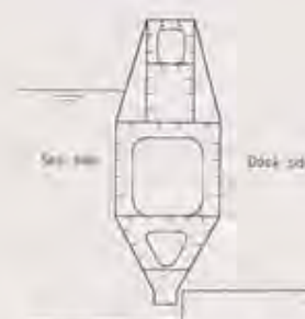
Fig. 1 Pontoon type gate
